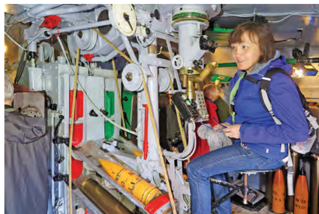
Elena at the controls of the 15cm twin barrelled gun at Stevns, originally built for the Gneisenau . The red and green correspond to port and starboard barrels, which could be controlled independently in elevation, but not in traverse. The separate cartridge and shell for the gun can be seen bottom left
